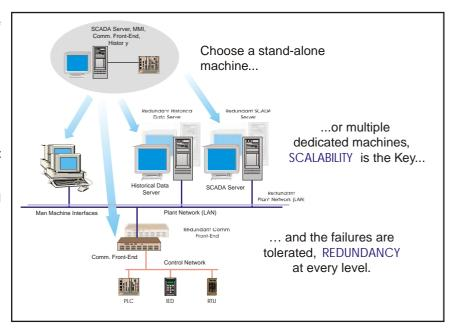
SIRIUS supports redundancy of the following which enables fault tolerant, high availability system architecture.
